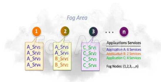
Fig. 1 (a). Application Services Placed on a Single Fog Node
