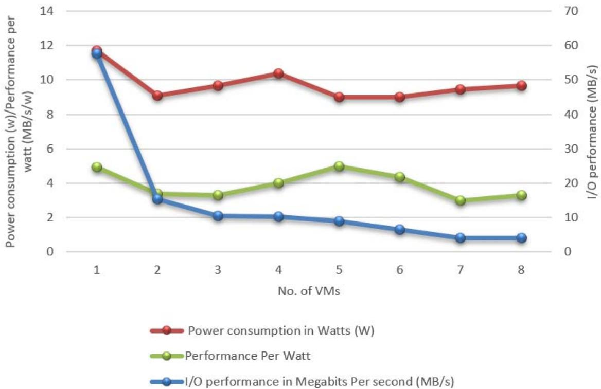
Fig. 3: The effect of increasing the number of VMs executing aio-stress on power consumption, power performance and I/O performance
