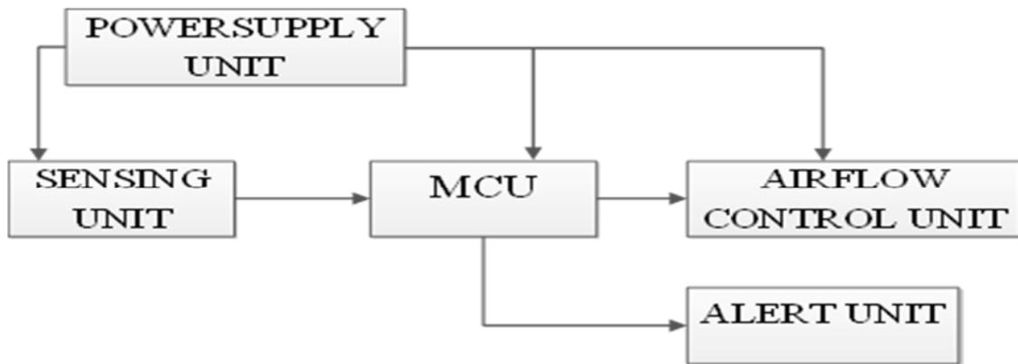
Fig. 1: Block Diagram of the CO Monitoring and Control System
