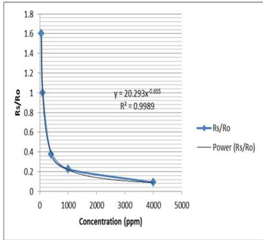
Fig. 5: Mathematical Modelling of Sensor Sensitivity Graph
