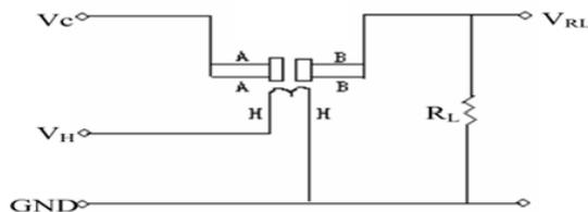
Fig. 6: Basic Loop Test of MQ-7 Sensor
