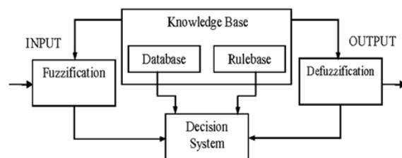
Fig.5 a Type-1 Fuzzy System Structure
