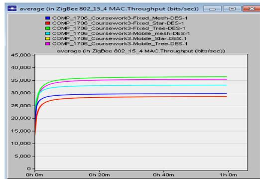
Fig. 15. MAC Throughput (Fixed Vs Mobile)
