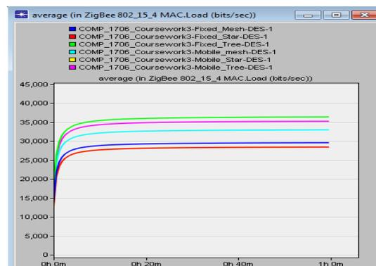
Fig. 13. Comparative MAC Load (Fixed Vs Mobile)
