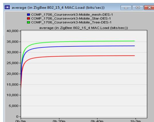
Fig. 10. MAC Load (bits/s) in Mobile Network
