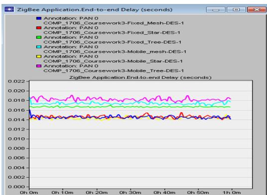
**Fig. 17. End-to-End Delay(s) (Fixed Vs Mobile)**
