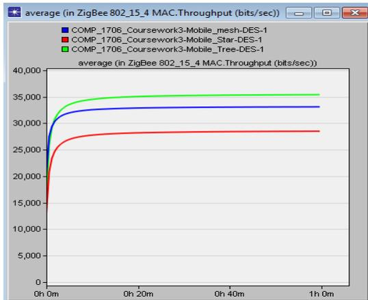
Fig. 11. Throughput in Mobile Network
