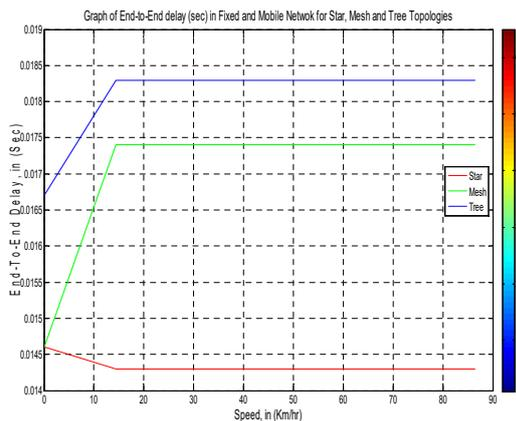
**Fig. 18. Graph End-to-End delay (sec) in Fixed and Mobile Network**
