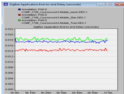
Fig. 12. End-to-End Delay (sec) in Mobile Network
