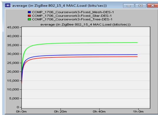
Fig. 7. MAC Load (bits/s) in Fixed Network
