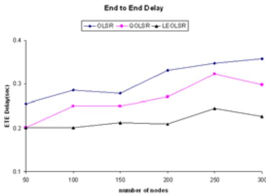
Figure 8. End-To-End Delay (sec) of data packets –Network Density.
