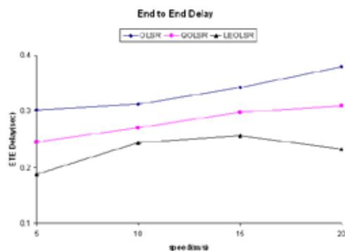
Figure5. End-To-End Delay (sec) of data packets - Network Mobility.
