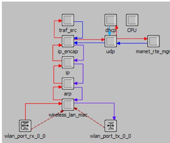
Figure 4. Node model of MANET station[9]
