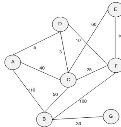
Figure3. Bandwidth-QoS Network Example for MPR Selection
