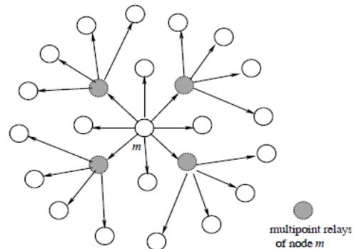
Figure1. Multipoint relays of node  $m$  [8]
