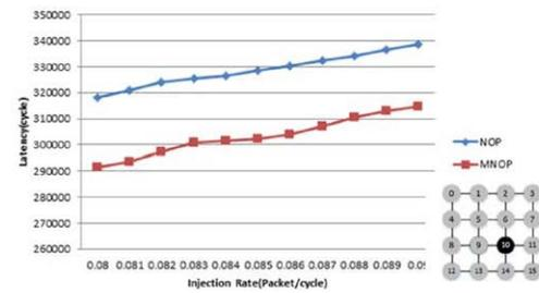
Fig. 5d. Latency result, when using West-first routing under Hotspot traffic pattern, node 10
