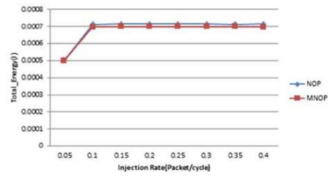
Fig. 5b. Energy result, when using North-last routing under Butterfly traffic pattern
