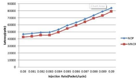
Fig. 5f. Latency result, when using West-first routing under Shuffle traffic pattern
