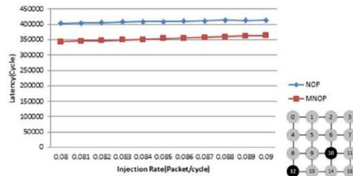
Fig. 5e. Latency result, when using West-first routing under Hotspot traffic pattern, nodes (10,12)
