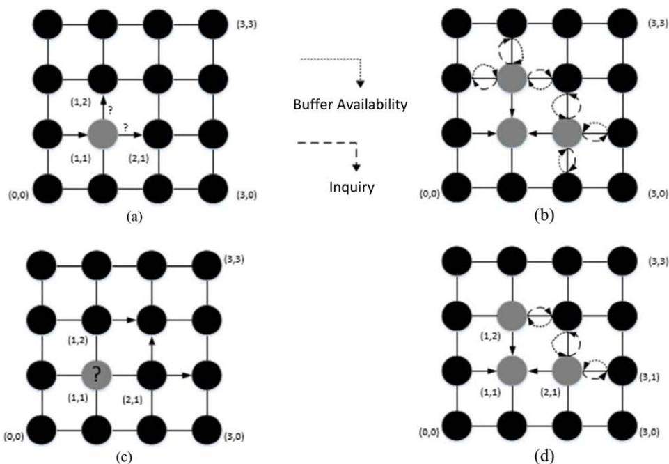
Fig .3. MNoP selection roadmap. a. Condition of hesitation. b. Input buffer availability and number of inquiries of non-adjacent nodes. c. Computation of the adjacent nodes. d. Using of the input buffer and inquiry status of MNoP to make the selection.
