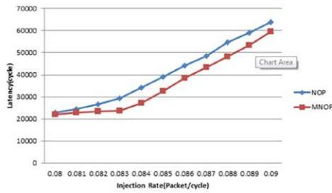
Fig. 5a. Latency result, when using North-last routing under Butterfly traffic pattern
