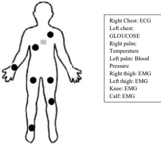
Fig. 1 The location of nodes on the body
