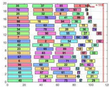
Figure 6: How tasks executed in the allocated machines along with execution time by LPT algorithm
